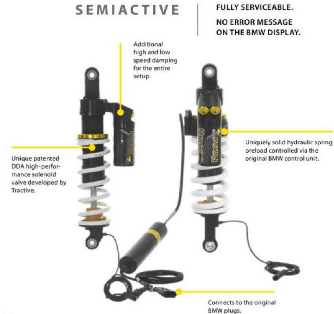
**The basic setup fitted here is designed for riders up to 100 kg including luggage.** Modifications are possible for a heavier rider (more than 100 kg) and/or if the bike is usually ridden with a passenger / with luggage. In this case, we individually modify the shock absorber to meet your needs by fitting a spring with a higher spring rate. Please fill out our suspension check form and send it back to us.
